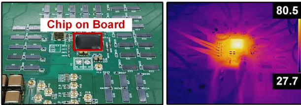
Fig. 9. PCB photo with 40 GaN transistors and thermal image in normal switching mode.
